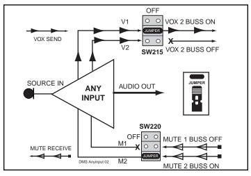
Fig. 8B - Any Input VOX 1 and MUTE 2 Activated
